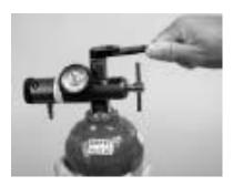
When not in use, close the cylinder by turning the wrench clockwise all the way.
